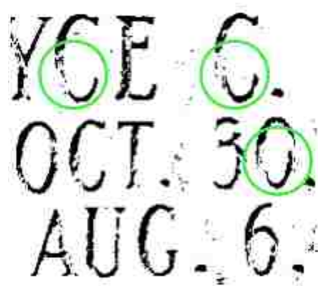
Figure 2.3: The text region of a noisy headstone after Sauvola binarization. The circles denote breaks in characters due to inconsistent contrast and coloration within
